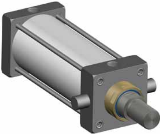
4" bore, 2" rod diameter, triple oversize Rod, with a one pcs steel head trunnion with cushion. ST3O3T1X-4X8-#2
